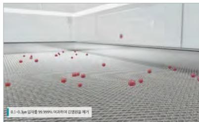
ULPA filter that removes 99.999% of 0.1~0.3 \mu\text{m} particles
